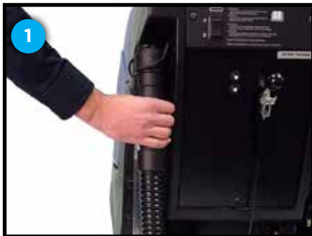
Recovery tank drain hose
