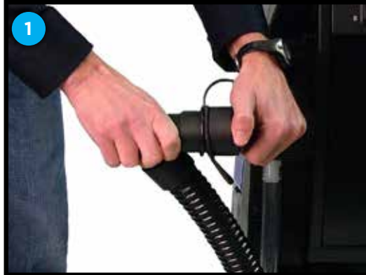
Check for clog in the restriction collar
