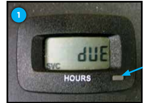
Hour meter showing "SVC DUE"
