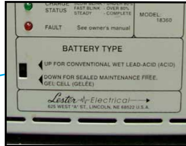
Close up of dip switch
