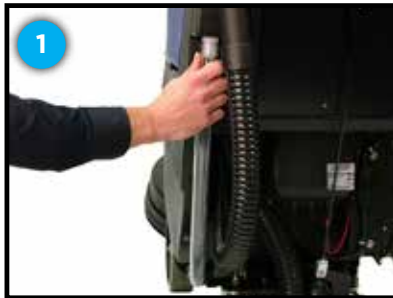
Check sight gage hose for solution level
