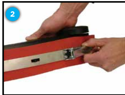
To flip or replace squeegee blades, release over-center latch
