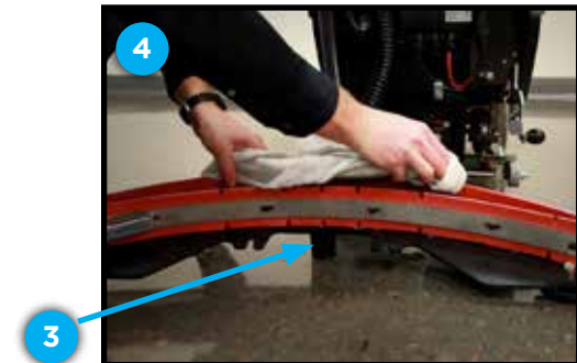
After checking for wear, wipe the blade or flip it to a new edge
