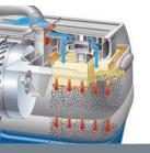
Filter cleaning: powerful pulses of air from above effectively clean the filter. The cleaning process is activated by a control on
