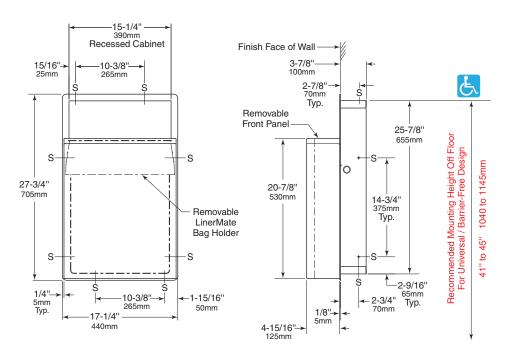
Rough Wall Opening 15-7/8" (405mm) wide 26-1/4" (665mm) high 4" (100mm) minimum recessed depth
