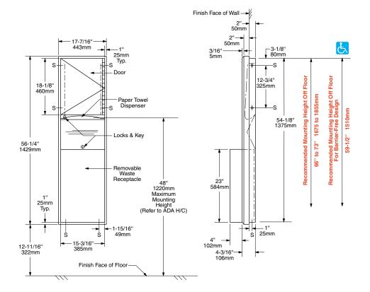
Rough Wall Opening 16" (406mm) wide 54-3/4" (1390mm) high 2-1/4" (57mm) minimum recessed depth
